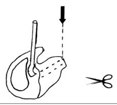
4. Cut the tapered tubing close as possible to the earmould. Any tube sticking out could rub your ear and make it sore.
