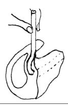
1. Pull the old tubing out of the earmould. Do not throw the old tubing away as you will need it later.
