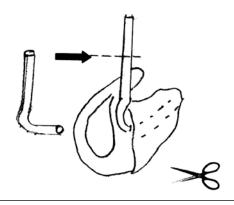
5. Take the old piece of tubing you saved and line it up with the newly threaded tube. Cut the end to the same length.
