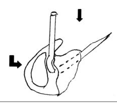
3. Pull the tube until the bend reaches the mould. All the tapered section should have come through the other side.
