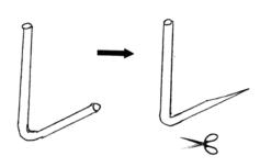
2. Cut the last 2 inches of a pre-bent piece of tubing to a tapered end. Thread this through the earmould until it comes out the other end.
