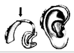
6. Push the end of the tubing onto the plastic nozzle on your hearing aid. Make sure that it bends in the right direction, as shown in the picture.
